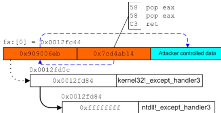
Figure 2.2: Gaining code execution from an SEH overwrite
