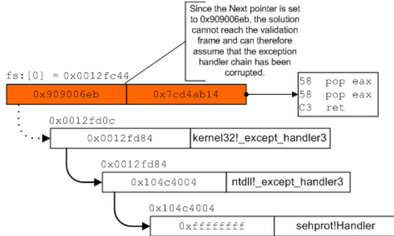
Figure 3.1: Detecting corruption of the exception handler chain
